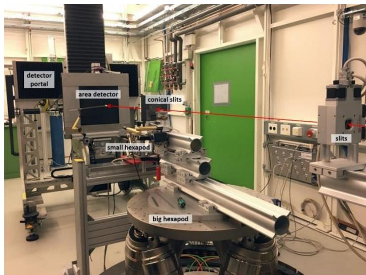
Figure 27 - P07 - EH3 with JJ X-ray slits, big hexapod, conical slit cell set-up and PE detector on the detector portal.
