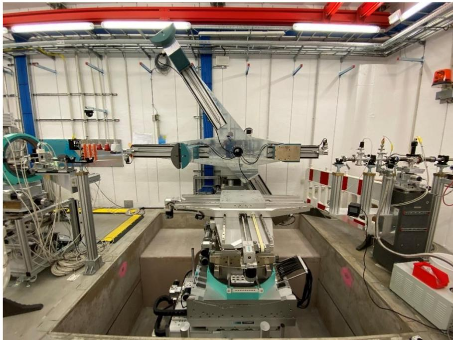
Figure 22 - Heavy load diffractometer at P61A.
