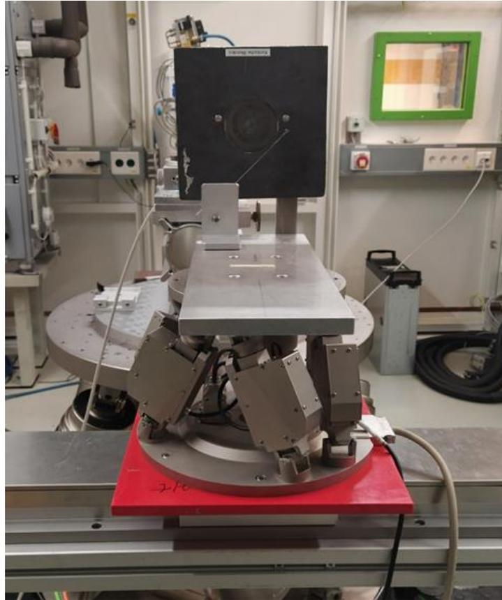
Figure 43 - View of the mini-hexapod together with the CSC attached to it.
